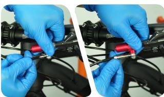
03. Tighten the Banjo Fixing Bolt using 4mm Hex wrench(Torque 4-6N⋅m)
