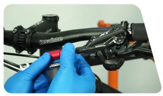
02. Tighten hex using 15mm spanner(Torque 4-6N·m).
