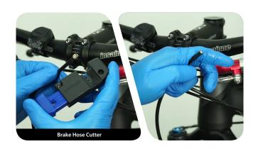
02. Remove the compression bolt from the brake hose.
