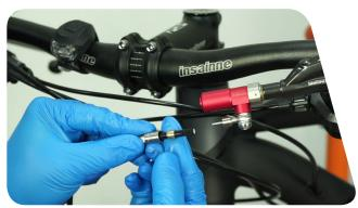
02. Join the Brake hose to the Insert until there is No gap between the hose and the banjo.
