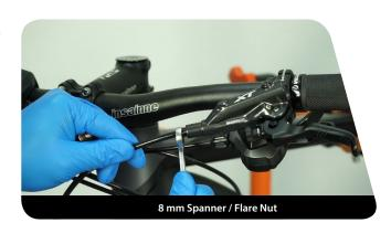
02. Remove the brake hose from the lever body.
