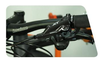
01. Loosen the compression bolt using 8mm spanner.
