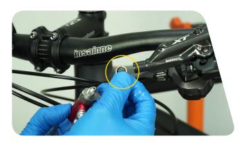
01. Thread Outbraker into the lever body by hand first.
